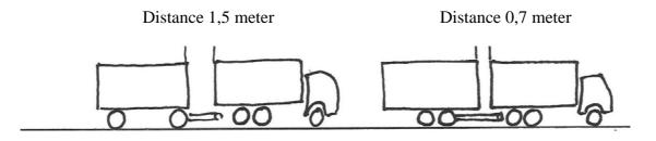
The safe version in Norway: Roadtrain of 19,5 meter with drawbar trailer
